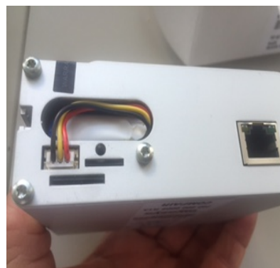
Insert and connect batteries
